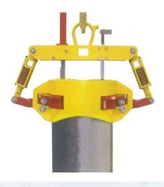
PATENTED BELL-PINCERS (ITEM 2): Enables the electrode or the electrode column to be picked up without a lifting plug. It can be safely used as an alternative to other electrode transport systems...., while maintaining the use of the safety latch on the crane hook.
