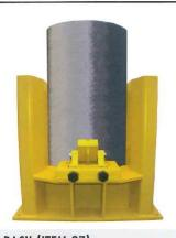
**ELECTRODE STORAGE RACK (ITEM 27):** Equipment to vertically hold and store electrode columns for prolonged periods of time. The electrode columns are held tight by eccentric locks manually positioned. The rack is welded or screwed by bolts to the floor. A special feature is access from the side to provide easier loading/unloading operations for the crane operator.
