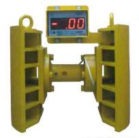
TORQUE METER FOR FURNACE CLAMPS (ITEM 28): Enables to check periodically the furnace clamps tightening strength. It becomes necessary when doing maintenance work at the furnace arms. A light and well designed tool, equipped with a display for the immediate read of the measured value.
