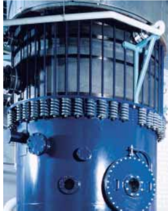
▲ Flue gas scrubbing with ®DIABON graphite pipe quencher (installed height 1.3 m approx.) mounted on a co-current scrubber. Liquid feed: to pipes at left, to cooling ring at top
